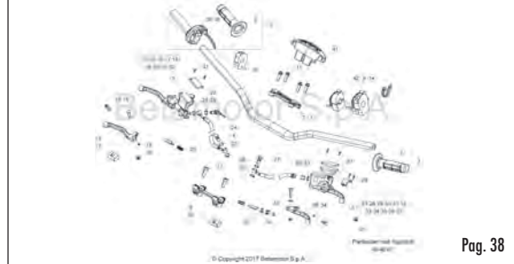
TAV.35 Comandi-Manubrio - Controls-Handlebars - Commandes-Guidon - Bedienungselemente-Lenker - Mandos-Manillar
